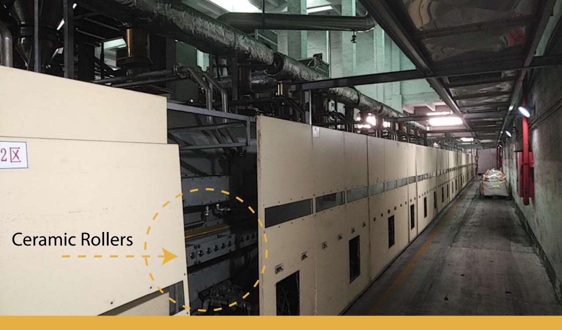
5-9 rollers / meter Heat resistant ceramic rollers array
